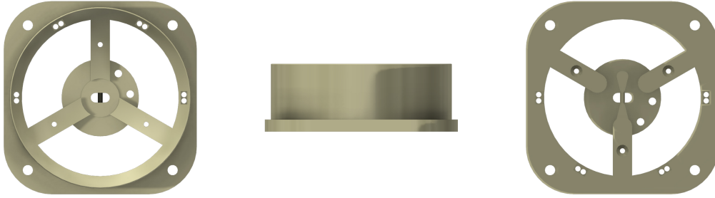
Figure 6.6: Bottom, side and top view of the MIRKA2 mounting platform version 2. From the top view the supporting structure for the polyethylene cord used to secure the MIRKA2 capsule can be seen. Three boreholes for the alignment pins, and two boreholes for the burn wire bolts can be seen in both the top and bottom views.
